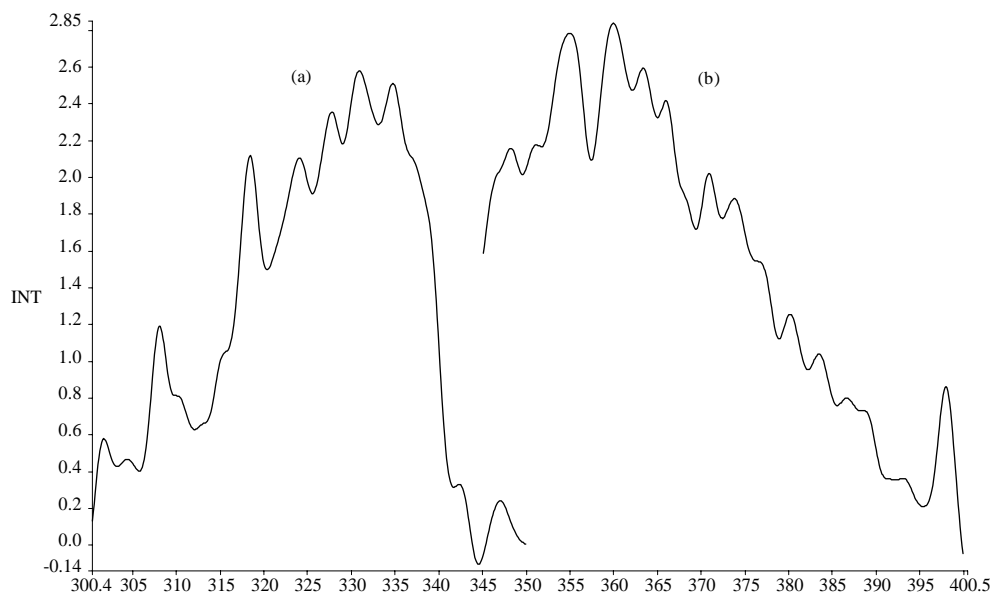
Fig. 6. Fluorescence excitation and emission spectra of the naphthoxazine functional poly( \epsilon -caprolacton) (PCL N-a) (P1 in Table 1, 6.5 g/l) in \text{CHCl}_3 . \lambda_{\text{exc}} = 335 \text{ nm} , \lambda_{\text{emis}} = 360 \text{ nm} .
